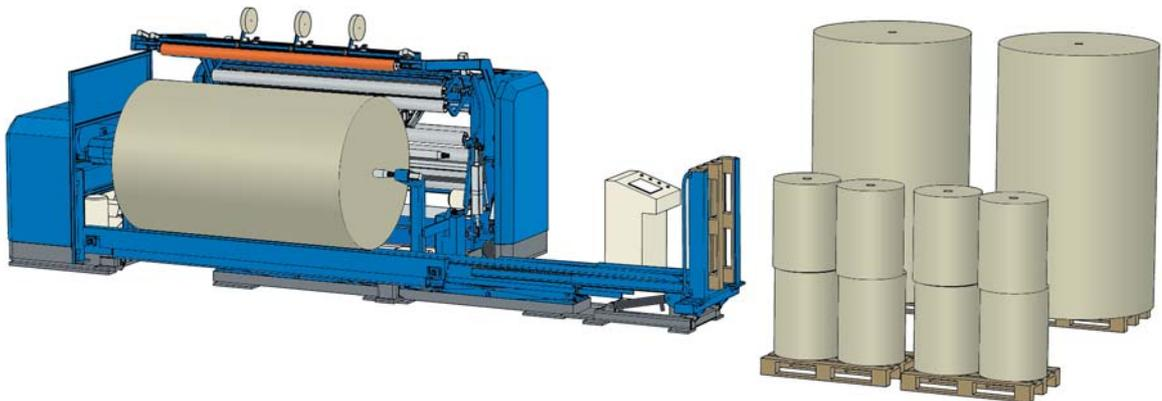
**The SFC 2533** is optimised for fast production of smaller, lighter rolls of single face corrugated. The SFC 2533 comes with a loading table onto which the finished rolls are ejected. For smaller web widths (max. 1800 mm) and where space is limited, the SFC 1833 is available.
