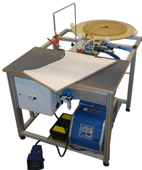
This machine is used when applying a plastic edge strip on Re-board® with hot-melt glue. The machine comprises a table on which the operator places the board that is to be supplied with an edging strip. The edge strip is then pressed securely onto the Re-board®
