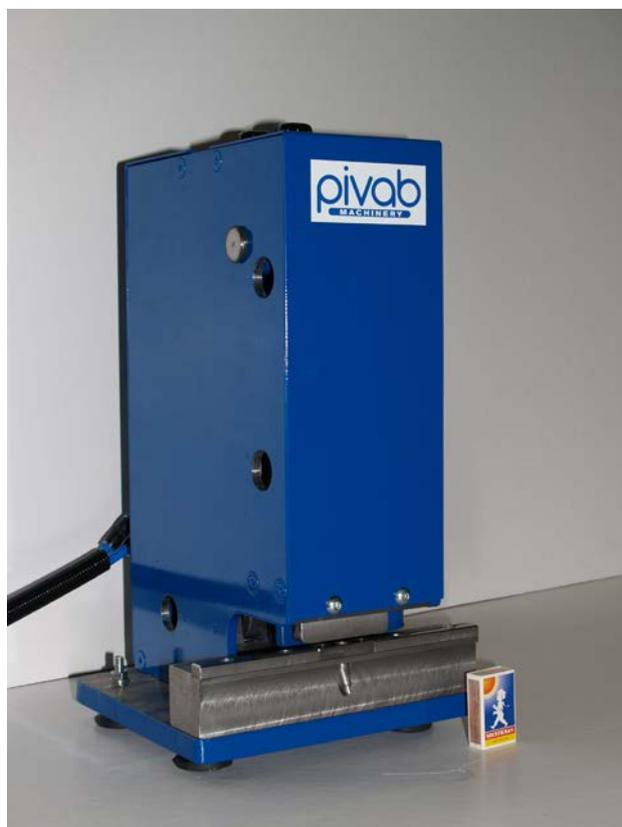
This is a machine which facilitates usage of different fasteners when using Re-board® in a number of different applications. It opens up a convenient way of applying Screws when there is a need for attaching boards together or other devices to a board. The punch is pneumatic driven unit controlled via a foot pedal. Easy change of internal punch tools with different shapes is one obvious advantage.
