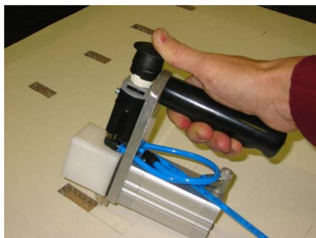
The partial pluckier tool is used for removing pieces of the board for insertions of connecting boards. It removes 50x16mm material at a time. The Pluckier tool is pneumatically driven so air supply is needed.
