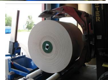
Loading – with overhead crane or clamp truck
