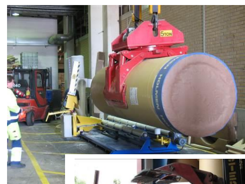
Loading – with overhead crane or clamp truck
