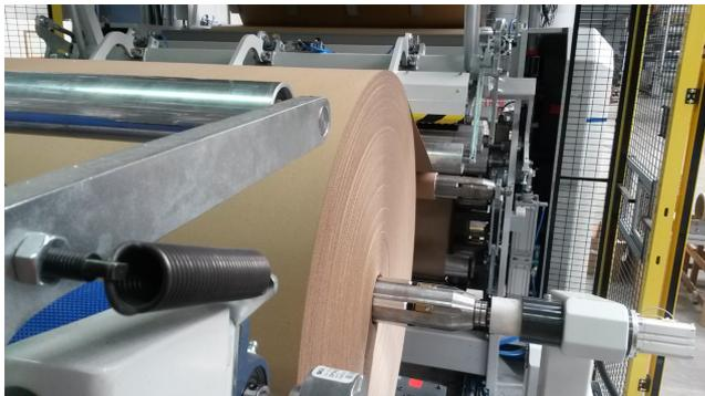
Fully automatic rewriter for single face corrugated board.
