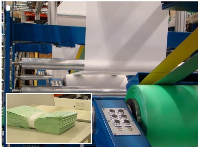
3 layers of material are laminated to form the bed sheet.
