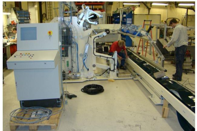
Single face rewriter in final production at Pivab's plant.
