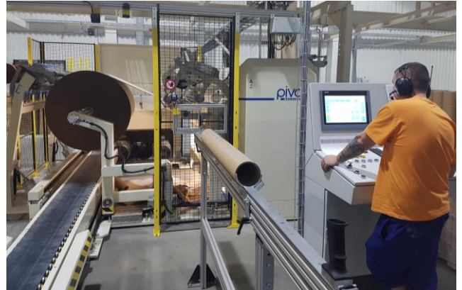
New installation of Pivab rewinder SFC 2583 1,8m at Dot2Dot, Poland.
